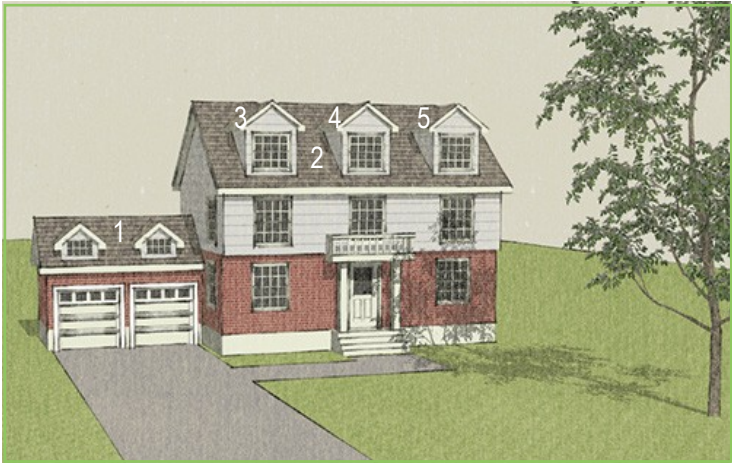
Figure 3.2.9.2 - Suitable - At least two (2) roof planes are visible from the public right-of-way.
