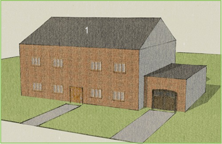
Figure 3.2.9.1 - Not Suitable - Only one (1) roof plane is visible from the public right-of-way.
